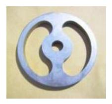
Here are two different spacer plates often called kidney plates. They serve the same function. Either a very course grind or a spacer for stuffing sausage.
