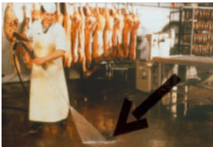
Fig. 469: Cleaning with pressurized water must be avoided in rooms where meat is present
