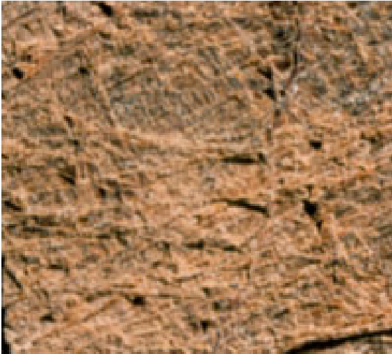
Fig. 485: Wooden cutting board, knife incisions close up when wet and imbed bacteria (hygienically not acceptable)
